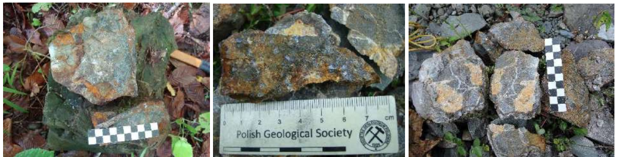
Figure 8. a. Altered rocks b. Fractures filled with galena, sphalerite and pyrrhotite c. Hydrothermal breccia
