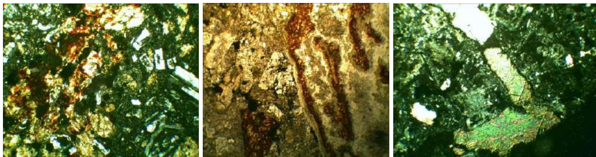
Figure 15. Photomicrographs of hydrothermally altered hyperthene basalt X40.
