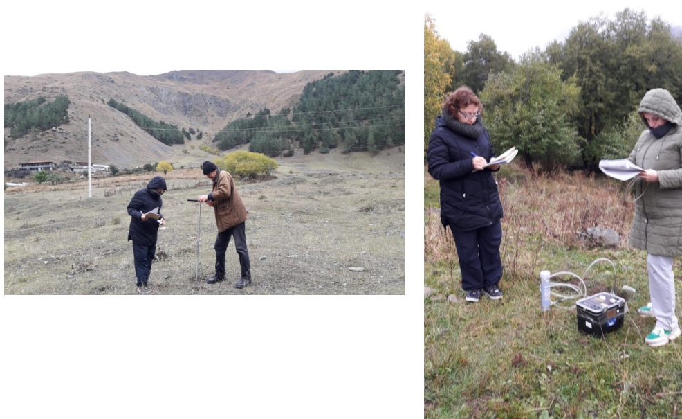
Figure 8. The process of measuring radon concentration in soil air
